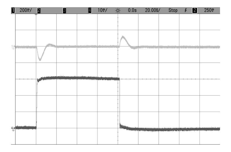
Figure 5. V<sub>OUT2</sub> Load Step Response
