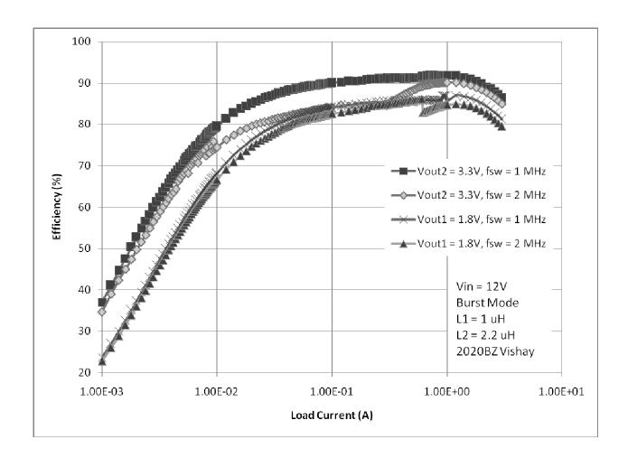
Figure 6. LTC3633A-3 DC1896 Efficiency
