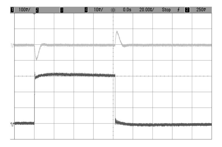
Figure 4. V<sub>OUT1</sub> Load Step Response
