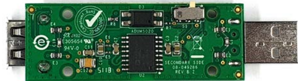
Figure 3. S1 Switch Position for Full Speed Operation
