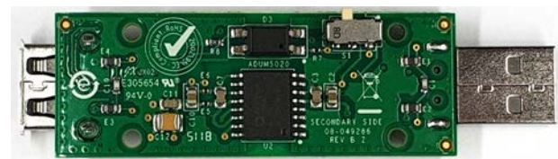
Figure 4. S1 Switch Position for Low Speed Operation
