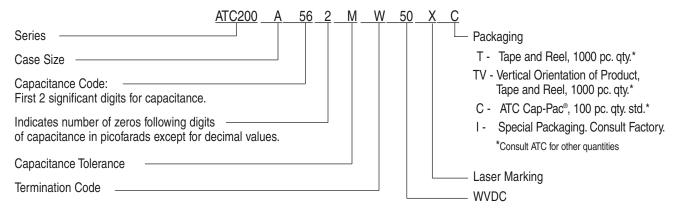
The above part number refers to a 200 A Series (case size A) 5600 pF capacitor, M tolerance (±20%), 50 WVDC, with W termination (Tin/Lead, Solder Plated over Nickel Barrier), Laser Marking and ATC Cap-Pac® packaging.
