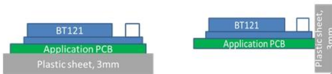
Blue curve Plastic sheet under antenna touching PCB
