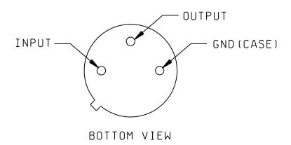
FIGURE 2. <u>Terminal connections</u>.
