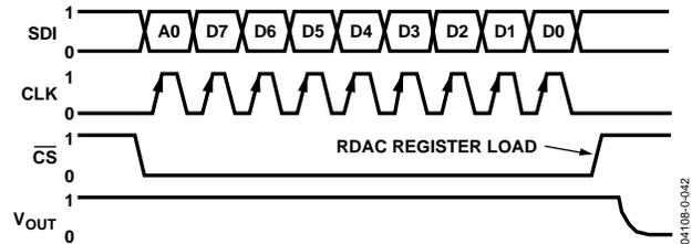
Figure 42. SPI Interface Timing Diagram
