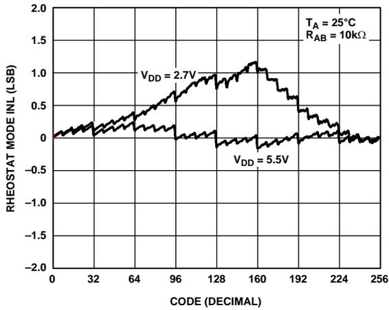
Figure 3. R-INL vs. Code vs. Supply Voltages
