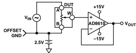
Figure 31. Test Circuit for Gain vs. Frequency
