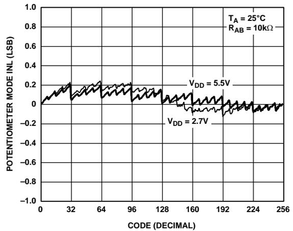
Figure 7. INL vs. Code vs. Supply Voltages
