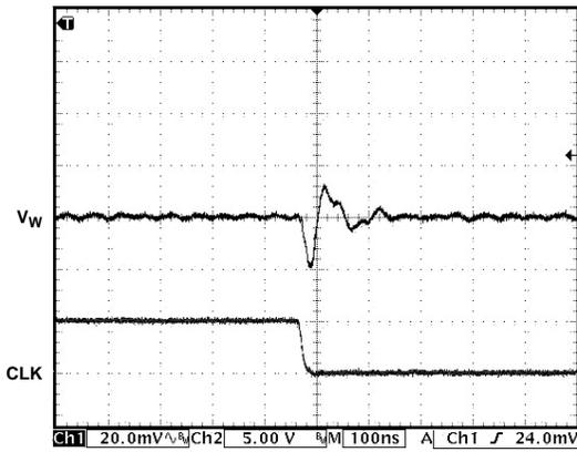
Figure 22. Digital Feedthrough
