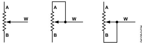
Figure 33. Rheostat Mode Configuration
