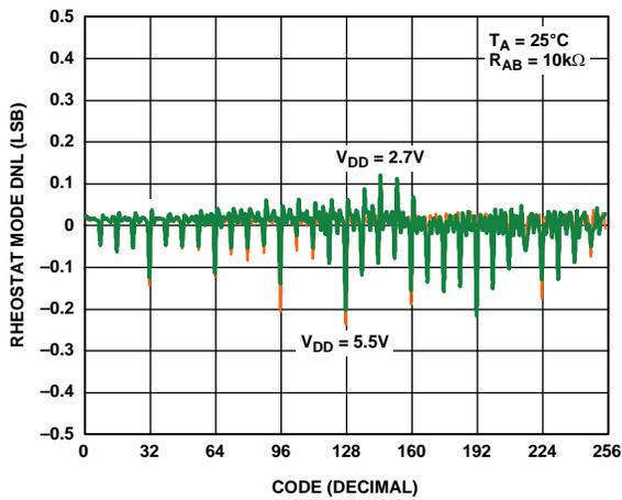
Figure 4. R-DNL vs. Code vs. Supply Voltages
