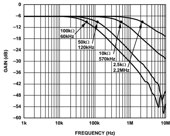
Figure 20. -3 dB Bandwidth at Code = 0x80
