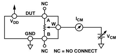
Figure 32. Test Circuit for Common-Mode Leakage Current
