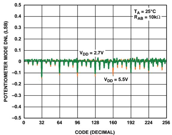
Figure 8. DNL vs. Code vs. Supply Voltages
