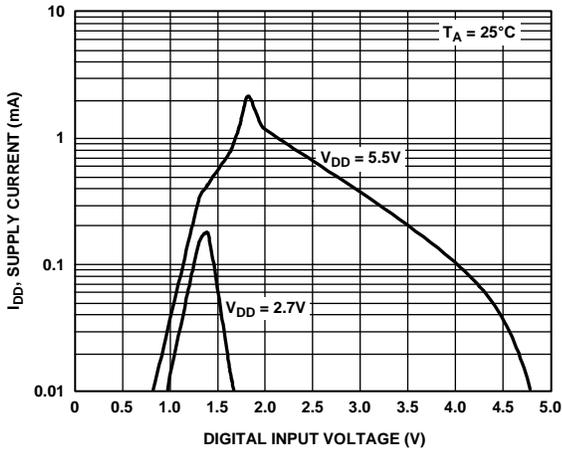
Figure 21. Supply Current vs. Digital Input Voltage
