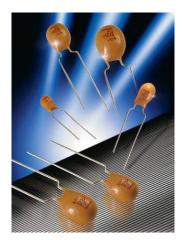
TAP is a professional grade device manufactured with a flame retardant coating and featuring low leakage current and impedance, very small physical sizes and exceptional temperature stability. It is designed and conditioned to operate to +125°C (see page 282 for voltage derating above 85°C) and is available loose or taped and reeled for auto insertion. The 15 case sizes with wide capacitance and working voltage ranges means the TAP can accommodate almost any application.
