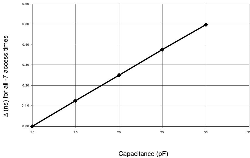
(b) Load Derating Curve
