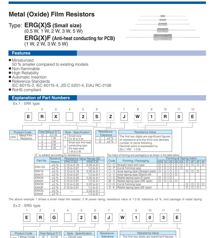
The above example 2 shows a small metal oxide film resistor, 2 W power rating, resistance value of 10 kΩ, tolerance ±5 %, and package of radial taping
