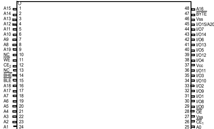
Figure 2. 48-pin TSOP I Pinout (Dual Chip Enable without ERR) – CY62167G [3, 4]
