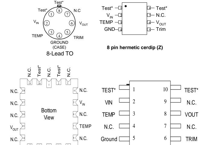
Figure 1 - <u>Terminal connections</u>.
