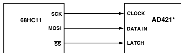
Figure 8. AD421 to 68HC11 Interface
