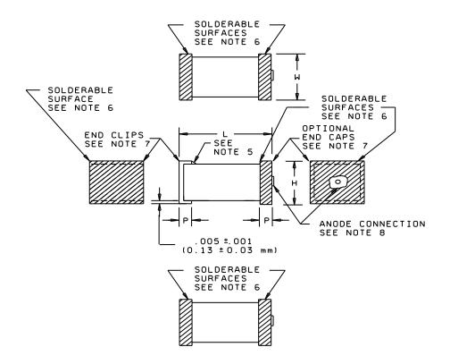
FIGURE 1. Style CWR06 (conformally coated) capacitors.
