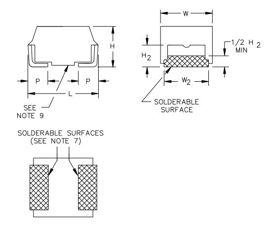
FIGURE 2. Style CWR09 (molded chip) capacitors.
