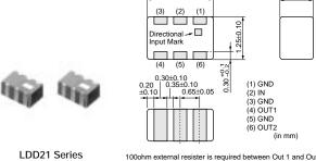
100ohm external resister is required between Out 1 and Out 2. All the technical data and information contained herein are subject to change without prior notice.
