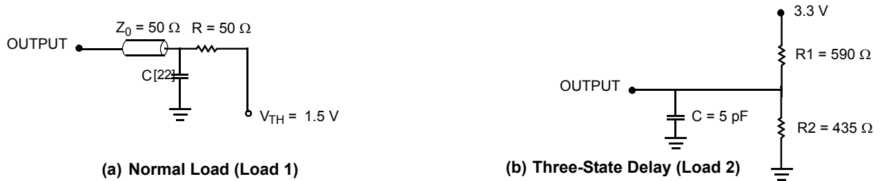
Figure 3. AC Test Loads and Waveforms
