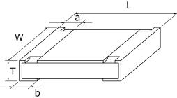
Unit: mm **Dimensions** Mass (Weight) Part No. W (g/1000 pcs) b ERJU2R 1.00±0.05  $0.50 \pm 0.05$  $0.20\pm0.10$  $0.25 \pm 0.10$  $0.35 \pm 0.05$ 0.8 ERJU3R 0.80+0.15/-0.05 0.45±0.10  $1.60 \pm 0.15$  $0.30\pm0.20$  $0.30 \pm 0.15$ 2 ERJU6R 2.00±0.20 1.25±0.10 0.40±0.20 0.40±0.20 0.60±0.10 4
