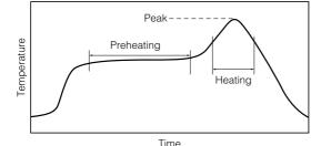
• Recommended soldering conditions for flow
