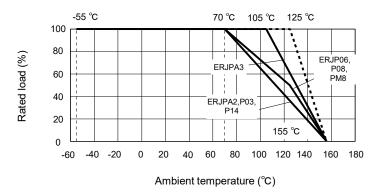
•For resistors operated in ambient rated terminal part temperature, power rating shall be derated in accordance with the figure below.
