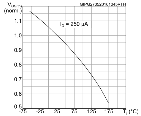
Figure 9: Normalized gate threshold voltage vs temperature
