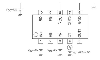
CT pin charge/discharge voltage (VCT)
