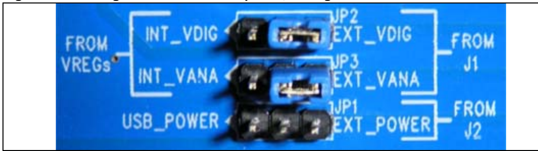
Figure 23. Configuration for external power, through J1
