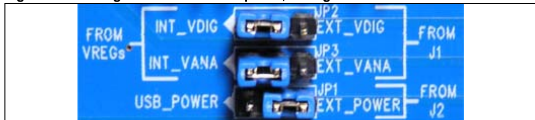
Figure 22. Configuration for external power, through J2
