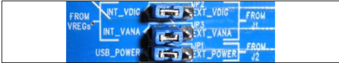
Figure 15. Configuration for supplying power through USB
