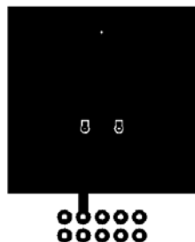
a) 40 ^{\circ}\text{C}/\text{W} when mounted on a 1 in 2 pad of 2 oz copper
