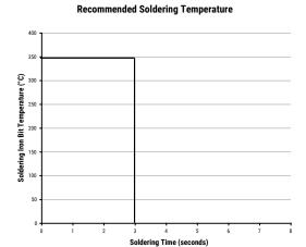
Soldering iron tip temperature should be set at 350°C (+10°C maximum) with the soldering duration not to exceed more than three seconds.
