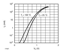
Fig. 1 - Forward Characteristics
