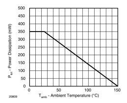
Fig. 3 - Admissible Power Dissipation vs. Ambient Temperature
