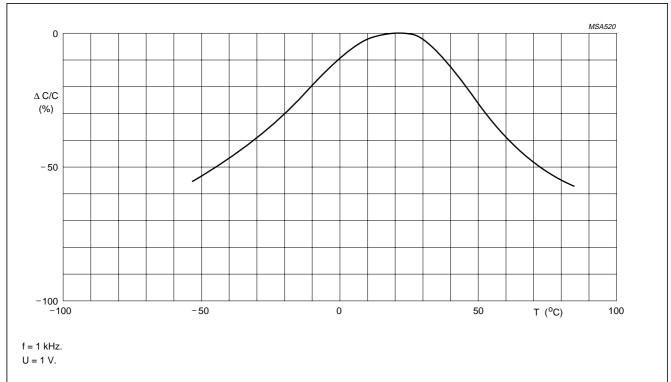
Fig.11 Maximum capacitance change with respect to capacitance value at 20 °C as a function of temperature.
