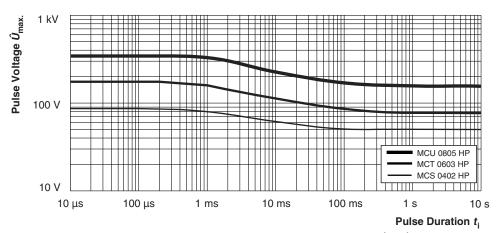
Maximum pulse voltage, single and continuous pulses; applicable if  $\hat{P} \leq \hat{P}_{\text{max}}$ ; for permissible resistance change ± (0.5 % R + 0.05  $\Omega$ )
