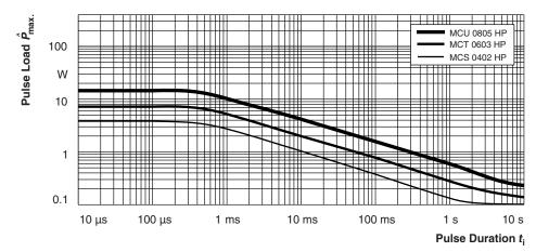
Maximum pulse load, single pulse; applicable if  $\overline{P} \to 0$  and n  $\leq$  1000 and  $\hat{U} \leq \hat{U}_{\rm max}$ ; for permissible resistance change  $\pm$  (0.5 % R + 0.05  $\Omega$ )
