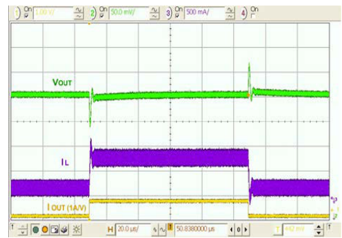
Figure 19. Load Transient, 200–800–200 mA, 100 ns Edge
