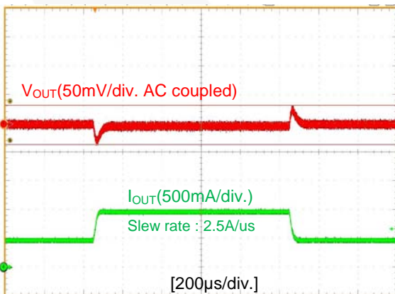
Figure 8. Load Transient Response(Step-up/down)
