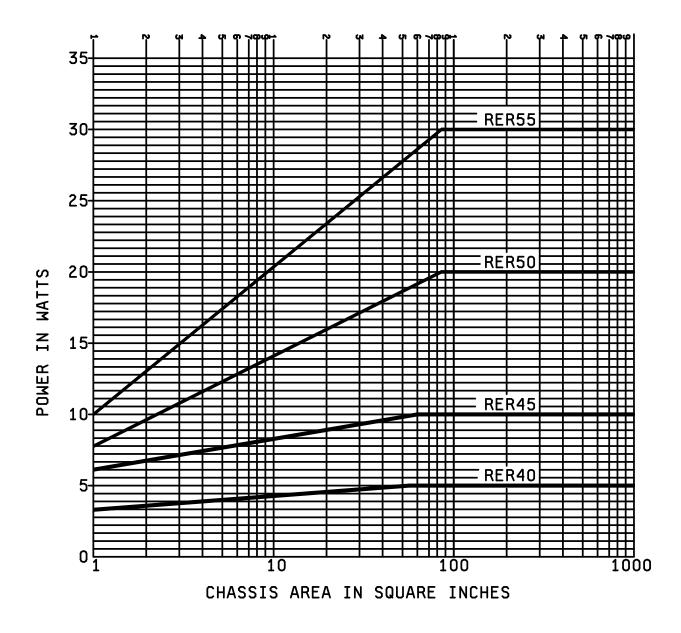
NOTE: The chassis derating curves are based on the full power ratings at an ambient temperature of 25°C. These curves are independent of the temperature derating curves.
