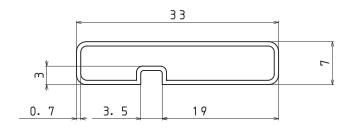
Tolerance=±0.3mm Thickness=0.7 $\pm$ 0.2mm Length =  $532.5 \pm 2$ mm Material = PVC (Antistatic treatment)
