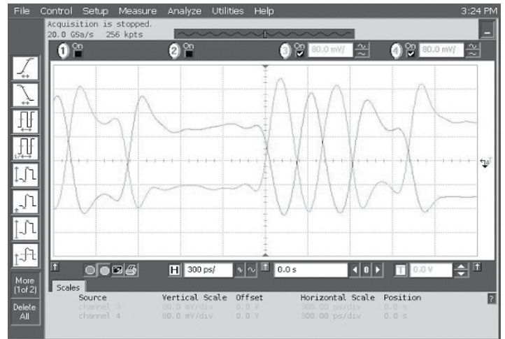
Data Waveforms, 2.5Gbps (left) & 5.0Gbps (right)
