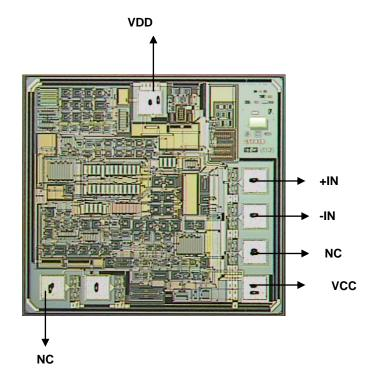
Die bonding pad locations and electrical functions
