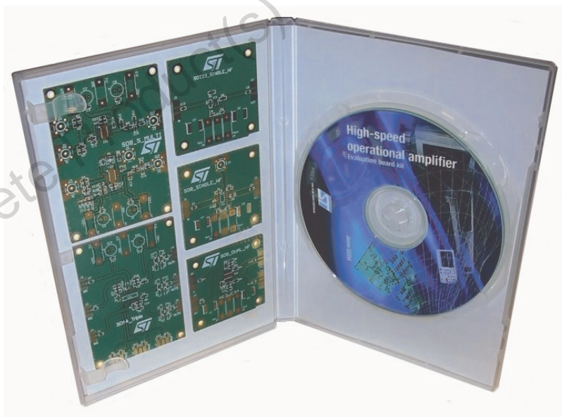
Figure 30. Evaluation kit for high-speed op-amps
