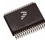
EK SUFFIX (PB-FREE) 98ASA10556D 32-PIN SOICW-EP
