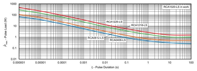
Maximum pulse load, single pulse; applicable if  $\bar{P} \to 0$  and n < 1000 and  $\hat{U} \le \hat{U}_{\text{max}}$ ; for permissible resistance change equivalent to 8000 h operation
