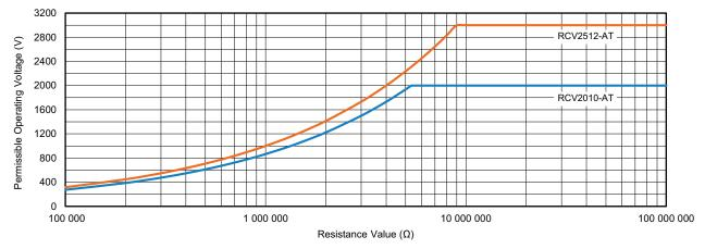
The permissible operating voltage  $U_{\rm max.}$  equals the rated voltage. For ambient temperatures above 70 °C power derating must be considered
