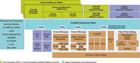
Core Complex (CPU, L2 and Frontside CoreNet Platform Cache) Basic Per Accelerators and Memory Control Networking Elements
