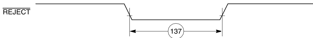
Figure 63. CAM Interface \overline{\text{REJECT}} Timing Diagram
