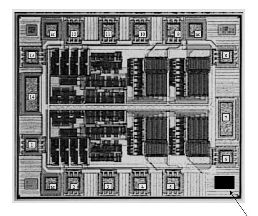
Pad size: Pad numbers 1 to 6 and 8 to 13: 100 x 100  $\mu$ m Pad numbers 7 (GND) and 14 (Vcc): 100 x 280  $\mu$ m
