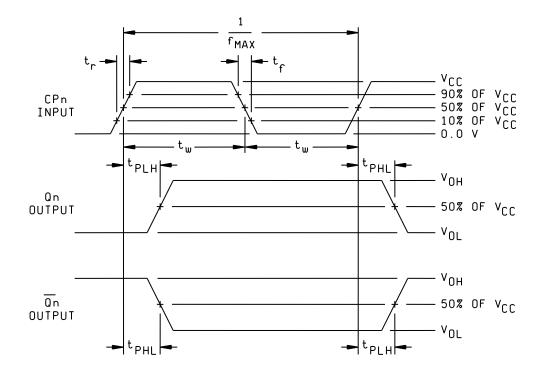
FIGURE 4. Switching waveforms and test circuit.
