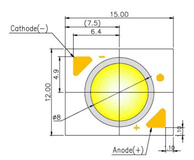
1. Unit: mm 2. Tolerance: ± 0.20 mm
