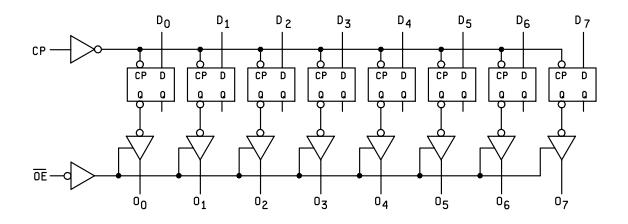
FIGURE 4. Logic diagram.
