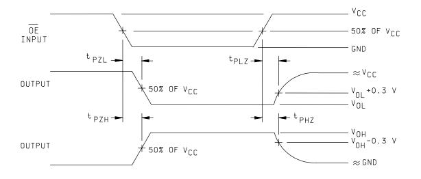
FIGURE 5. Switching waveforms and test circuit.
