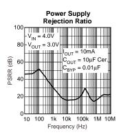
Power Supply Rejection Ratio vs. Voltage
