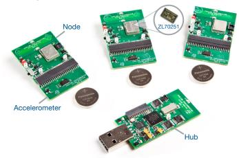
The included Z-Star protocol stack software supports Carrier Sense Multiple Access (CSMA) transactions in a star configuration. This robust, proprietary protocol is optimized for ultra-low-power wireless sensor networks and minimizes both packet size and transaction time. The protocol stack may be further optimized for specific customer applications (for example, by varying packet length, latency, and frequency of transmission).
