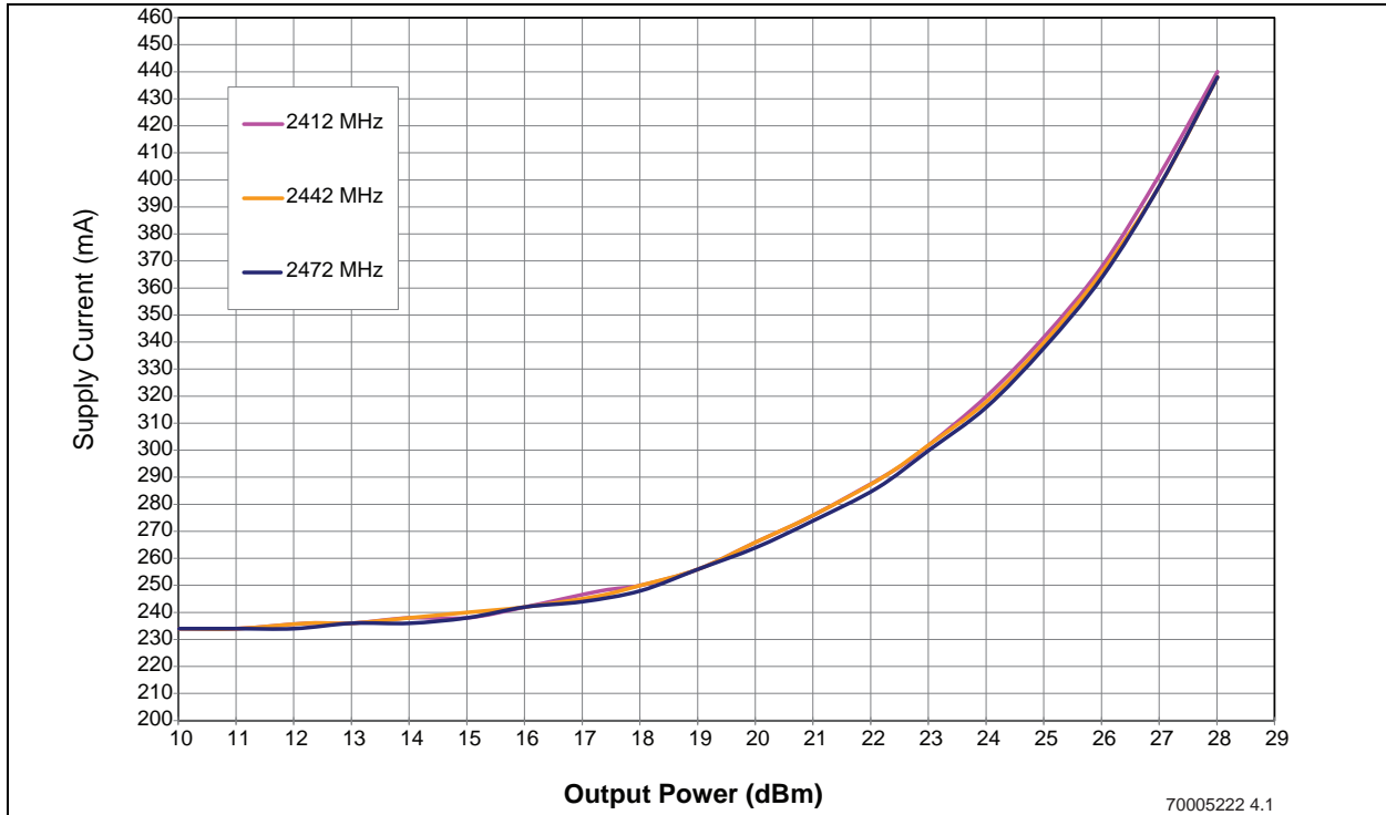
FIGURE 5-5: DC CURRENT VERSUS OUTPUT POWER
