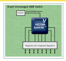
With its unique low power dissipation the VSC7388 enables fan less operation and thereby provides for higher system reliability and lower noise, both to the benefit of the user.
