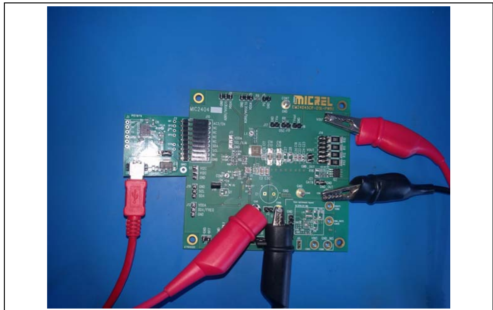
FIGURE 2-1: MIC24045 with MCP2221 Board Connection.
