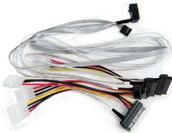
The Adaptec I-rA-HDmSAS-4SAS-SB-.8M is an internal right-angle mini SAS HD x4 (SFF-8643) (4) x1 Serial Attached SCSI (SFF-8482, adapter based) fan-out cable with sideband signals. It measures .8 meters and is used for connecting a Series 7/7Q/7H/7He adapter to SAS disks.
