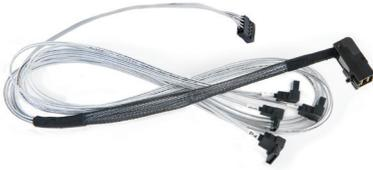
The Adaptec I-rA-HDmSAS-4rASATA-SB-.8M is an internal right-angle mini SAS HD x4 (SFF-8643) to right-angle (4) x1 Serial ATA fan-out cable with sideband signals. It measures .8 meters and is used for connecting a Series 7/7Q/7H/7He adapter to SATA disks, or a SAS/SATA backplane.
