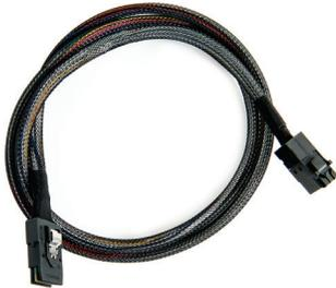
The Adaptec I-HDmSAS-mSAS-1M and .5M are internal mini SAS HD x4 (SFF-8643) to mini SAS (SFF-8087) x 4 cables. They measure 1 or .5 meters and are used for connecting a Series 7/7Q/7H/7He adapter to a SAS/SATA backplane with mini SAS HD connectors.
