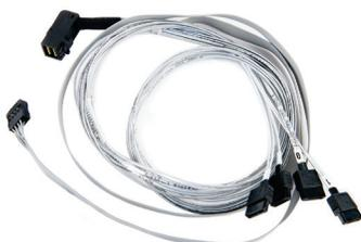
The Adaptec I-rA-HDmSAS-4SATA-SB-.8M is an internal right-angle mini SAS HD x4 (SFF-8643) to (4) x1 Serial ATA (adapter based) fan-out cable with sideband signals. It measures .8 meters and is used for connecting a Series 7/7Q/7H/7He adapter to SATA disks, or a SAS/SATA backplane.
