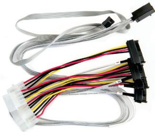
The Adaptec I-HDmSAS-4SAS-SB-.8M is an internal mini SAS HD x4 (SFF-8643) to (4) x1 Serial Attached SCSI (SFF-8482 adapter based) fan-out cable with sideband signals. It measures .8 meters and is used for connecting a Series 7/7Q/7H/7He adapter to SAS disks.
