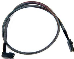
The Adaptec I-rA-HDmSAS-mSAS-.8M and .5M are internal right-angle mini SAS HD x4 (SFF-8643) to mini SAS (SFF-8087) x4 cables. They measure .8 or .5 meters and are used for connecting a Series 7/7Q/7H/7He adapter to a SAS/SATA backplane with mini SAS HD connectors.
