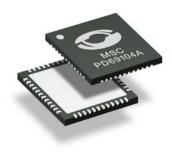
PD69104A is a 4-port, mixed signal, high-voltage High Power over Ethernet (HPoE) power sourcing equipment (PSE) manager. The IC enables the detection of IEEE802.3at-2009 Type 1 and Type 2 powered devices, ensuring safe power feeding and removal over Ethernet ports. It offers full digital control or fully autonomous operation in Auto mode with direct LED driving including a PoE MAX LED output. The PD69104A is ideal for 4-port Ethernet switches and requires a minimum of external components.
