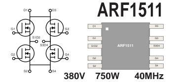
The ARF1511 is four RF power transistor arranged in an H-Bridge configuration. It is intended for off-line 300V operation in high power scientific, medical and, industrial RF power generator and amplifier applications up to 40 MHz.
