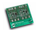
The MCP73837/8 AC/USB Dual Input Battery Charger Evaluation Board comes with a 10-pin DFN MCP73837 and a 10-pin MSOP MCP73838 pre-installed. The different packages can be easily evaluated by replacing the device, a resistor and a LED where the patterns have been pre-designed on the board layout.
